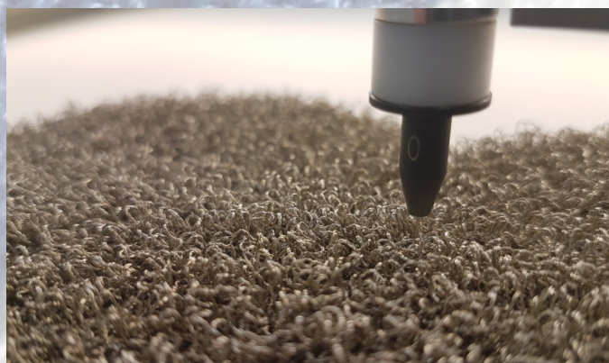
Moss embroidery with high loop density with the ZSK K-head
