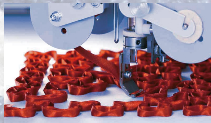
Ribbon embroidery with lateral fixation of the ribbon
